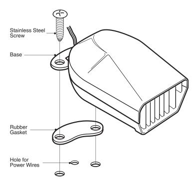
Insert mounting screws through base and the supplied rubber gasket. Use #10 stainless screws to fasten horn to deck. Apply marine sealant to horn base and wire hole.
